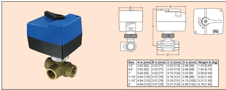
**The Series 3HBAV** is an electrical ball valve ideal for flow control in hot and cold water HVAC systems. These valves are typically used in conjunction with air conditioning systems, heating systems, water treatment and production industries. The 3HBAV is electrically driven open and/or closed via a bidirectional AC motor. The electrical valve offers a detachable actuator with position switches and indicator. The 3HBAV is available with modulating or floating actuators.
