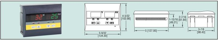
Simultaneously measure and control temperature and humidity with the Series THC Temperature/Humidity Switch. The unit offers a 3-digit red display for temperature indication and a 3-digit green display indicating humidity. The Series THC is equipped with four independent relays, two for temperature control and two relays for humidity control.
