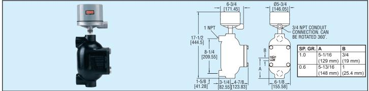
Flanged inspection plate allows periodic inspection and clean-out of Model 102 float chamber, making this unit ideal for use in refineries, chemical plants, and other areas with potentially dirty liquids. Low cost cast iron chamber is standard. Carbon steel and SS chambers are available on special order. SS float is standard.
