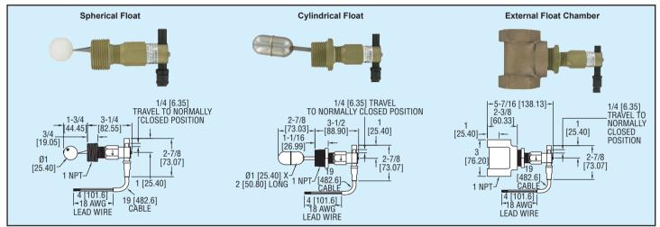
The Mini-Size Series L10 Flotect® Level Switches combine low cost with top quality materials and construction for great value and years of reliable liquid level control. Wide media compatibility is assured with a choice of brass or SS bodies and external tees; polypropylene or SS floats. Two basic configurations are offered; with 1" male NPT threads for direct side mounting through a half coupling or with factory installed tee for external mounting.
