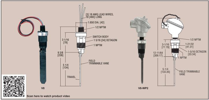
V8 Flotect® Flow Switch Protects Equipment: Operation is simple and dependable. In most applications, the switch is normally off while there is sufficient flow of liquid or air. When flow stops, the vane spring moves the vane, actuating a single pole double throw switch rated 5A @ 120/250 VAC to start or stop motor, pump, engine, etc. Operate a damper or valve; shut down a burner or actuate an alarm or signal, protecting unattended equipment from damage or loss of production.
